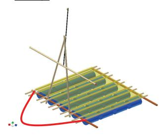
The rope needs to be between 8 and 10m long and tied securely to both corners of the bow, forming a loop. The rope should be a thick (min 25mm) nylon or manilla rope.
